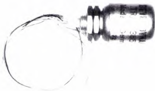
Fig. 1. Miniature audio transformer which provides gain in amplifiers developed for balanced-to-ground audio console.
