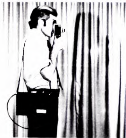
Miniature camera can be used with wireless transmitter to transmit pictures up to one hundred feet.
